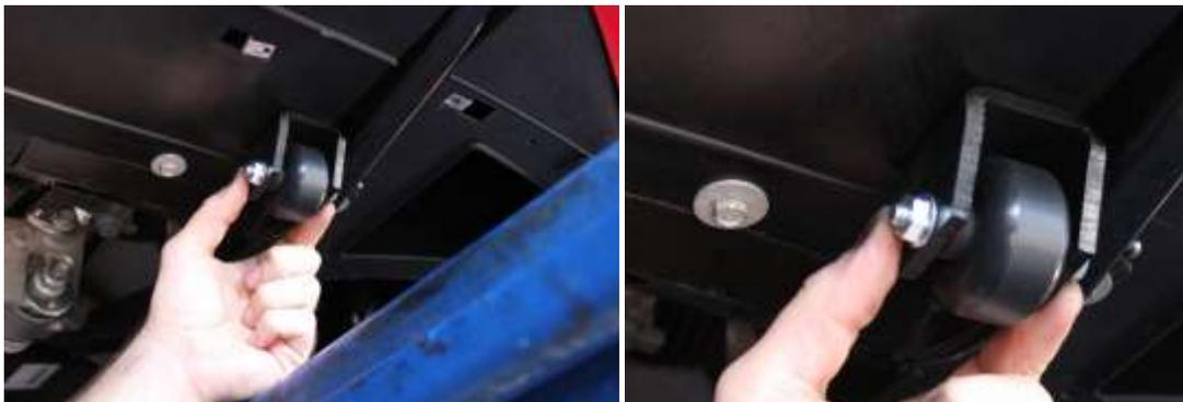
3. Bumper Savers are to be mounted to both insides of the lower radiator support arms so repeat this step on the other side (inside of support on left and right) as well.
