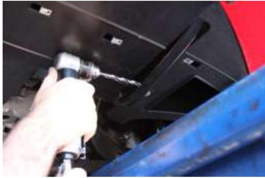
5. Press completed assemblies with 5/16 welded bolt through newly drilled holes as shown in picture and tighten bolts to compression.
