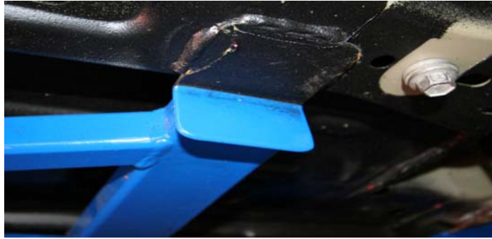
Above you will find a sample of the welded tab
