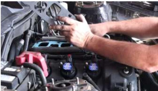
13. Place the .400" plenum spacer on top of the gasket and again ensure the patterns line up.
