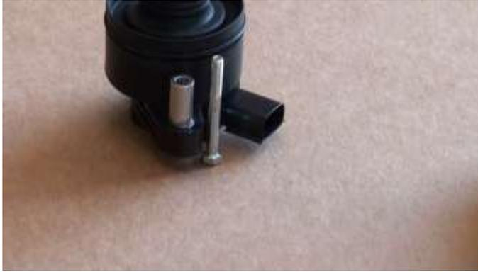
11. Insert your new Granatelli coils into place. You will note the gap between the mounting surface of the coil and the valve cover. Insert one of the supplied spacers in this gap and fasten with one of the long supplied bolts. Use the same 7mm socket to retighten to a snug fit. No need to ratchet down on the coils.
