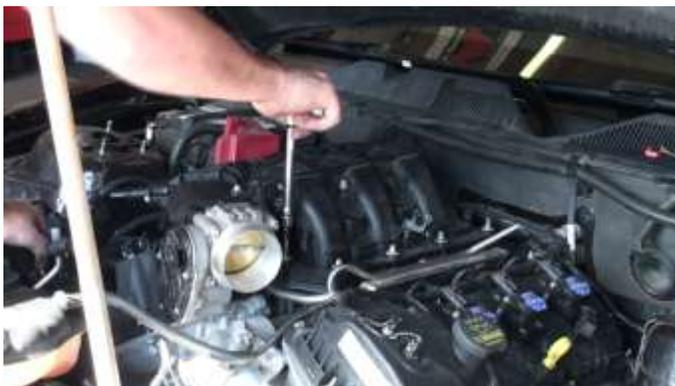
16. Reconnect all hoses and wiring harnesses that were removed.
