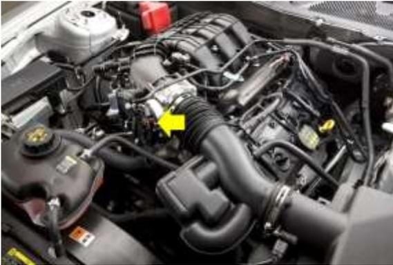
7. Remove all vacuum lines and wiring connections going to the upper plenum (intake manifold)
