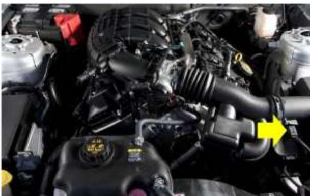
4. Remove the hose clamp that holds the rubber bellows from the air box to the throttle body.
