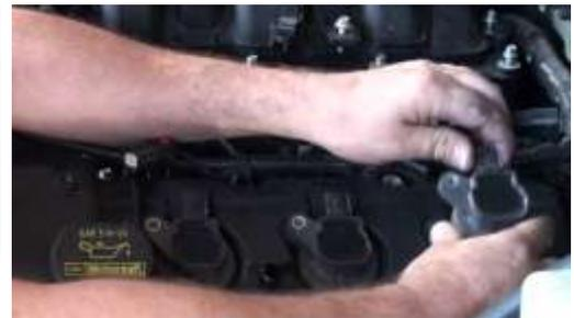
10. Your new Granatelli coils include a specifically designed spacer that allows for the higher capacity coils to work properly. Therefore, it requires one each (per coil) the supplied metal spacer and longer bolt.
